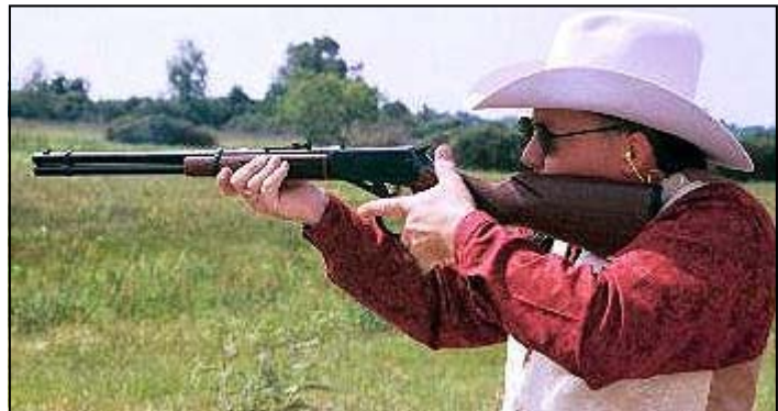
Rossi-built '92 carbine. The 19" ROUND barrel and band-mounted front sights mark it as a carbine instead of a Short Rifle.
